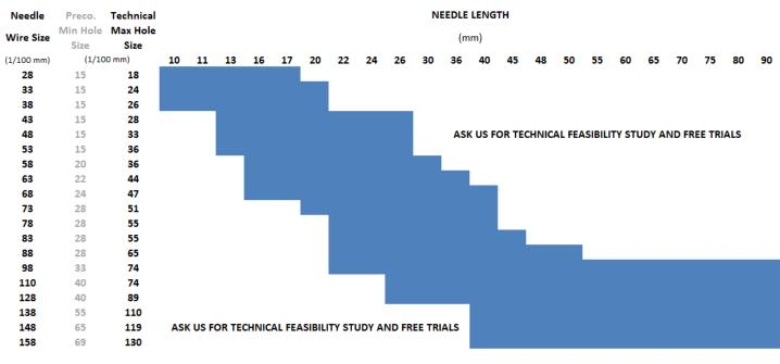
Available drilled-end sizes : 15 -18 - 20 - 22 - 24 - 26 - 28 - 31 - 33 - 36 - 40 - 44 - 47 - 51 - 55 - 59 - 61 - 65 - 69 - 74 - 79 - 84 - 89 - 93 -103 - 110 - 119 - 123 - 130 REQUEST US FOR DRILLING "DEEP"
